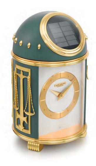
In 1954, Patek Philippe patented its extraordinary photoelectric energy mechanism (Patent No. 298564). Photoelectric cells charged an accumulator which then powered a motor to wind a conventional Patek Philippe 17''' hand-wound pocket watch movement. With energy stored in either the accumulator or the movement spring, the firm claimed that the clock was capable of running in complete darkness for a year and with an accuracy of within one second per day.
