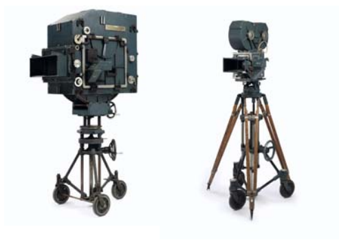
A three-strip Technicolor Camera (first picture shows the 'blimp' used to keep the camera "studio quiet") Estimate: £8,000-£12,000
